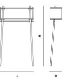
DIMENSIONS L 1120 x D 380 x H 2000 mm L 44 x D 14.9 x H 78.7 "
