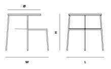
**DIMENSIONS** L 510 x D 600 x H 510 x Ø 450 mm L 20 x D 23.6 x H 20 x Ø 17.7 "
